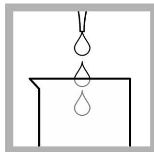
**4.** Use a TenSette Pipet to add 1.0 mL of Blanking Reagent to the beaker. Swirl to mix. The Blanking Reagent removes chlorine and chloramines from the water. **Note:** Use this solution in step 11.
