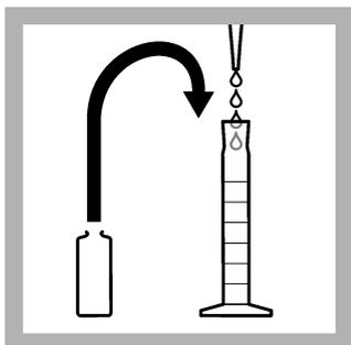
9. Use a TenSette Pipet with a clean tip to add 1 mL of indicator from the ampule to the same mixing cylinder.
