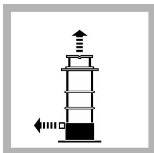
**18.** Pull the barrel valve button out to the "open" position. Pull the plunger up to separate it from the barrel assembly. Discard the remaining unfiltered sample. A new membrane may be necessary for very turbid samples. Alternatively, use a second Quick Filter unit with a new membrane filter installed.
