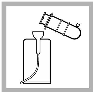
**22.** Pour the filtered, reacted sample from the plunger reservoir into the Pour-Thru Cell.
