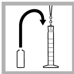
7. Use a TenSette Pipet with a clean tip to add 1 mL of buffer from the ampule to a clean and prepared 50-mL mixing cylinder.
