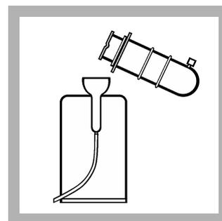
**16.** Pour the filtered, unreacted sample from the plunger reservoir into the Pour-Thru Cell.
