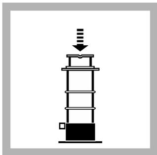
**21.** Insert the plunger into the barrel and slowly push the plunger down with even pressure, until the plunger is fully seated.
