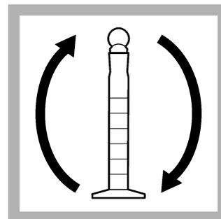
12. Put the stopper on the mixing cylinder. Invert the mixing cylinder two times to mix.
