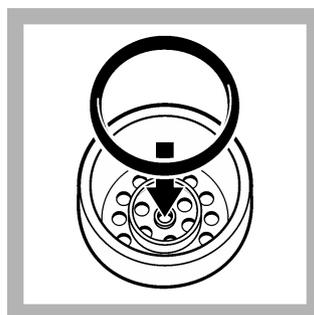
3. Remove the cap from the OriFlo plunger assembly. Make sure that the O-ring is seated correctly in the cap.
