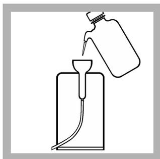
**2.** Flush the Pour-Thru Cell with at least 50-mL of deionized water.
