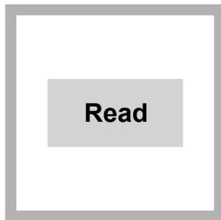
**23.** When the flow stops, push **READ**. Results show in  $\mu\text{g/L Cl}_2$ . If the sample contains a dechlorinating agent (e.g. sulfite or sulfur dioxide), the sample result (corrected for the reagent blank) will read "0" or a slightly negative value.
