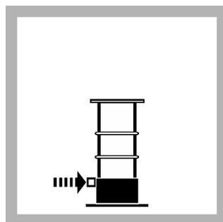
**19.** Push the barrel valve button to the "closed" position. Put the barrel assembly into its stand.
