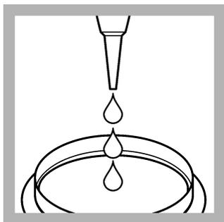
1. Invert one m-ColiBlue24 broth ampule 2 to 3 times. Open the ampule. Lift the lid of a petri dish and carefully pour the contents equally on the absorbent pad.
