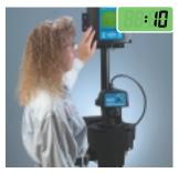
2. Place instrument head assembly on the ICE-PIC<sup>™</sup> Module. Wait for reading to stabilize (depends on instrument signal averaging setting) and verify that instrument is reading the ICE-PIC<sup>™</sup> Module within specification.
