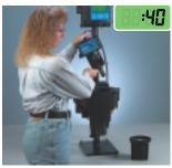
3. Remove the ICE-PIC<sup>™</sup> Module from instrument and replace head assembly on turbidimeter body. The instrument comes back on line automatically.
