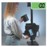
Set AquaTrend® Interface to "Hold Output" if required. Remove instrument head assembly and dry photocell window and optics mount with a soft cloth. Place the ICE-PIC™ Module in turbidimeter body.
