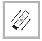
8. Remove the cap and add the contents of one SulfaVer 4 Sulfate Reagent Powder Pillow to the sample cell. Tighten the cap and invert to mix.
