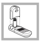
**10.** Within five minutes after the timer beeps, put the prepared sample in the instrument. Put the instrument cap over the sample cell.
